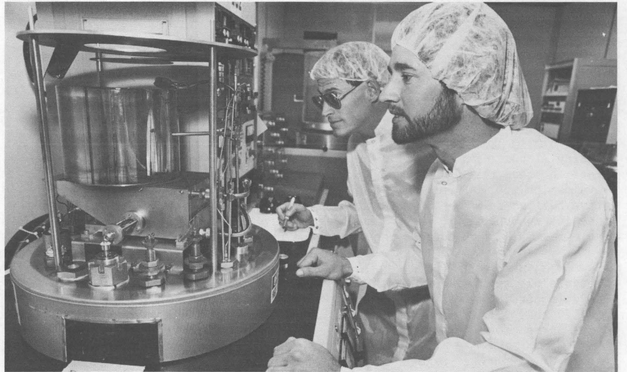
"GROWING" SUPERCONDUCTING thin films on a substrate with an electron-beam evaporator are Tom Zipperian (back) and Thomas Plut (both 1141). Electron-beam evaporation deposits thin films by directing a high-energy electron beam onto a material, which heats and evaporates the material, causing atoms to leave it and be deposited onto the substrate.
